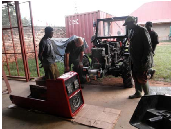
Fitting works of cable winch on the BFA-Tractor which was sent to Tanzania by Franz Rauch. The loading bridge was also produced in the Metal Workshop of VTC Mdabulo.
