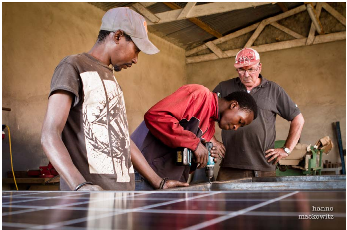
The steel frame for fixing the panel is made in the metal workshop of the VTC headquarter Mdabulo
