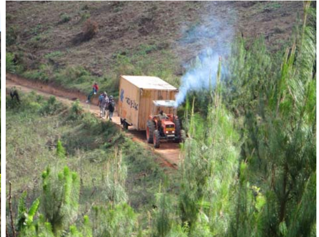
e) Container II was transported from the mission to the RDO plot with the help of a specially prepared wheel axle, which was put on the the tractor
