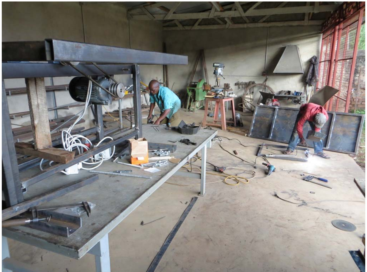
Prototype "for future products from the metal workshops Mdabulo (left foreground - an unfinished table saw, on the right- steel doors, etc. for Power House)
