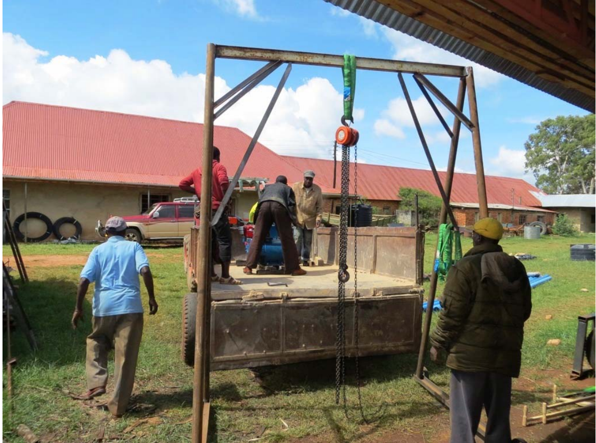
For the loading of the generator own elevator was built by Hannes Rauch
