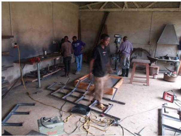
Shelving for material storage areas are produced in the Metalworking – Workshop
