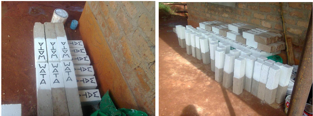
Fig. Concrete piles to mark the water lines in the terrain
